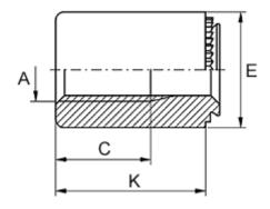
Female thread A = M5Height K = 24Min distance to edge = 4.0Outer diameter E = 9Plate thickness = 1.1 to 1.4
